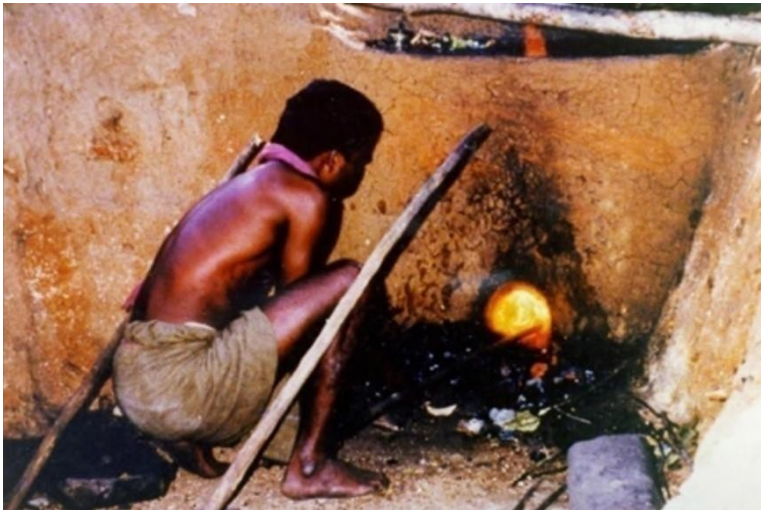
An underground furnace at Ghatgaon (Madhya Pradesh), with a tribal smelting iron ore. (Courtesy: A.V. Balasubramaniam)
